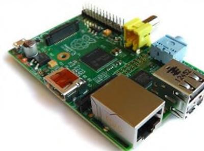
Gambar 2.4 Raspberry Pi Model B
