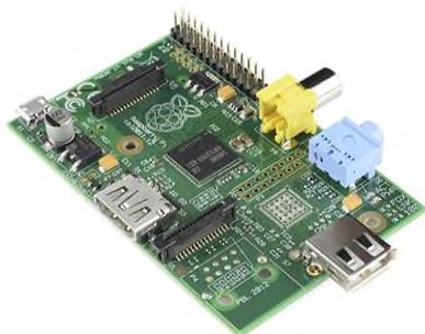
Gambar 2.2 Raspberry Pi Model A
