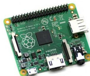
Gambar 2.3 Raspberry Pi Model A+
