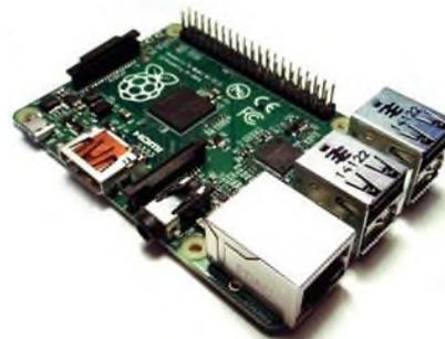
Gambar 2.5 Raspberry Pi Model B+
