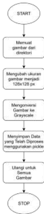
Gambar 2. Diagram Alur Program Preprocessing Data
